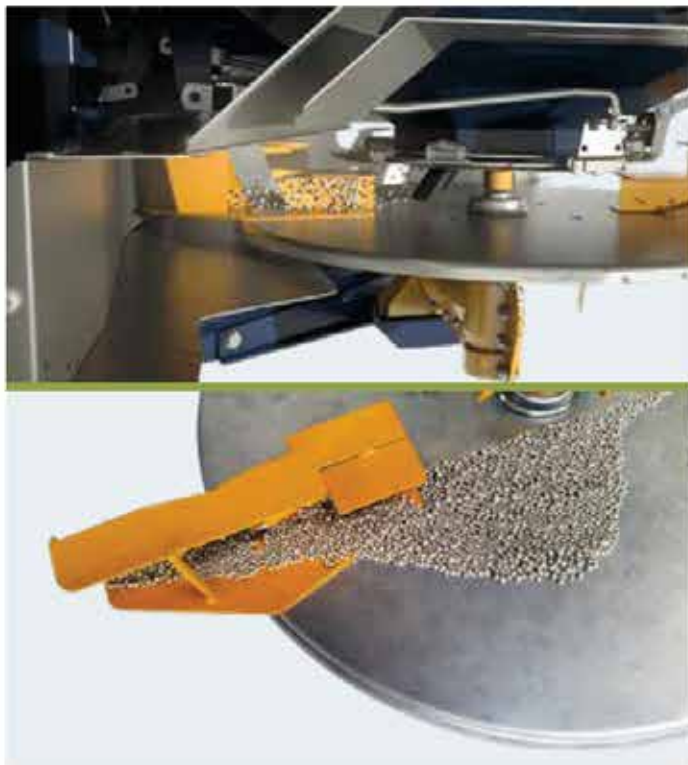
The large and flat spreading discs releases the fertiliser evenly on a 180 degree area.
