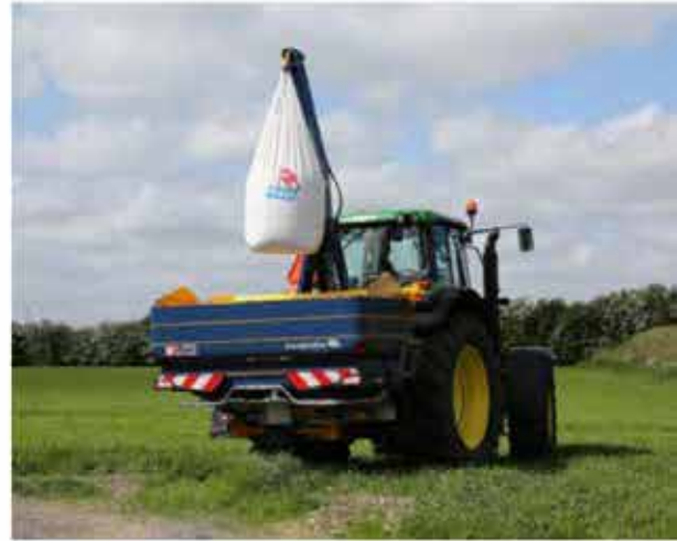
BXL 1300 can lift up to 1300 Kg and can be fitted on spreaders up to 3300 litres.
