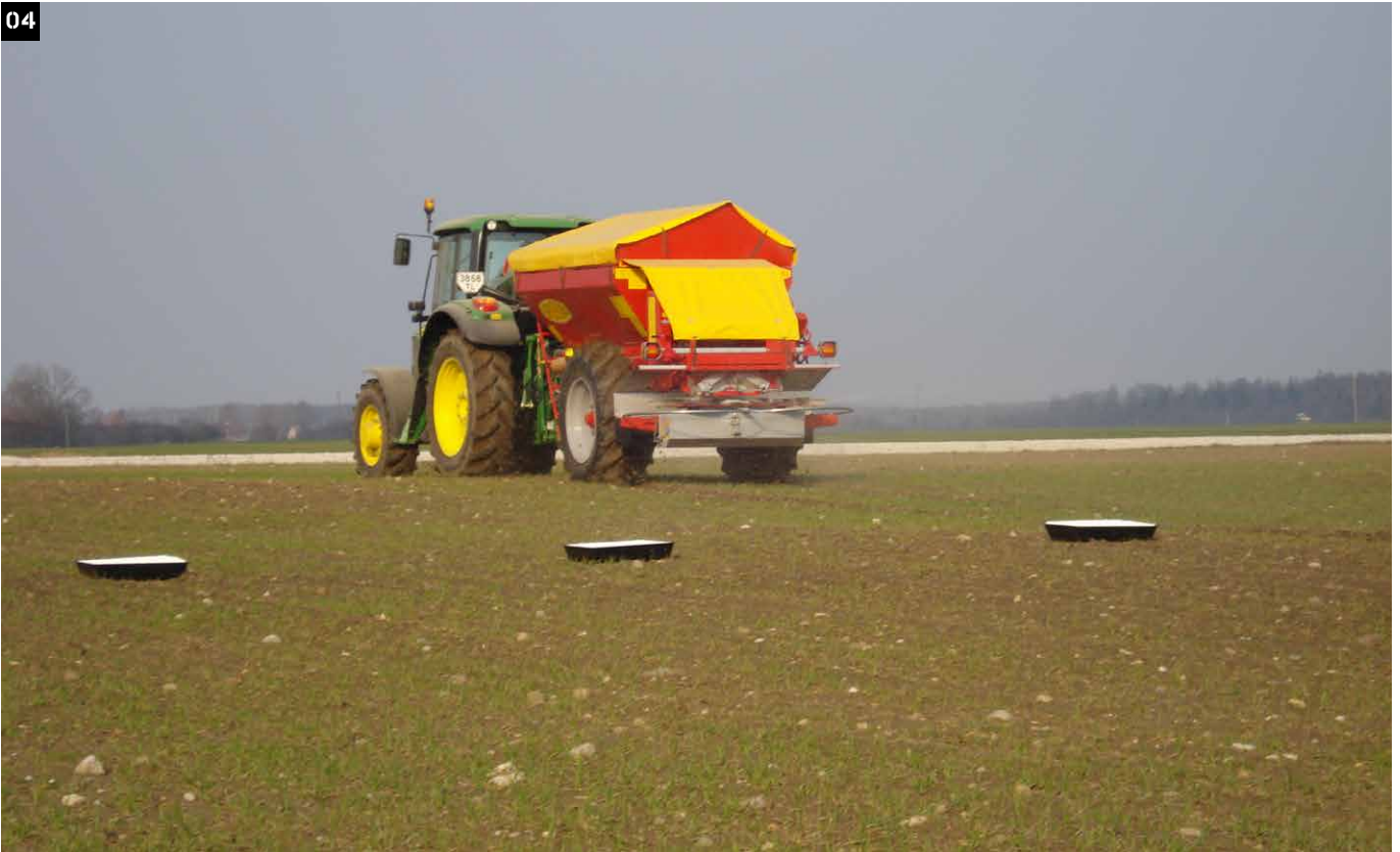
1 > A SIEVE TO MONITOR GRAIN SIZES 2 > MEASURING TUBE TO CONTROL SPREADING TEST RESULTS 3 > CALIBRATION KIT 4 > SPREADING TEST IN THE FIELD WITH Bredal K-spreader and Test kit (trays positioned on the field)
