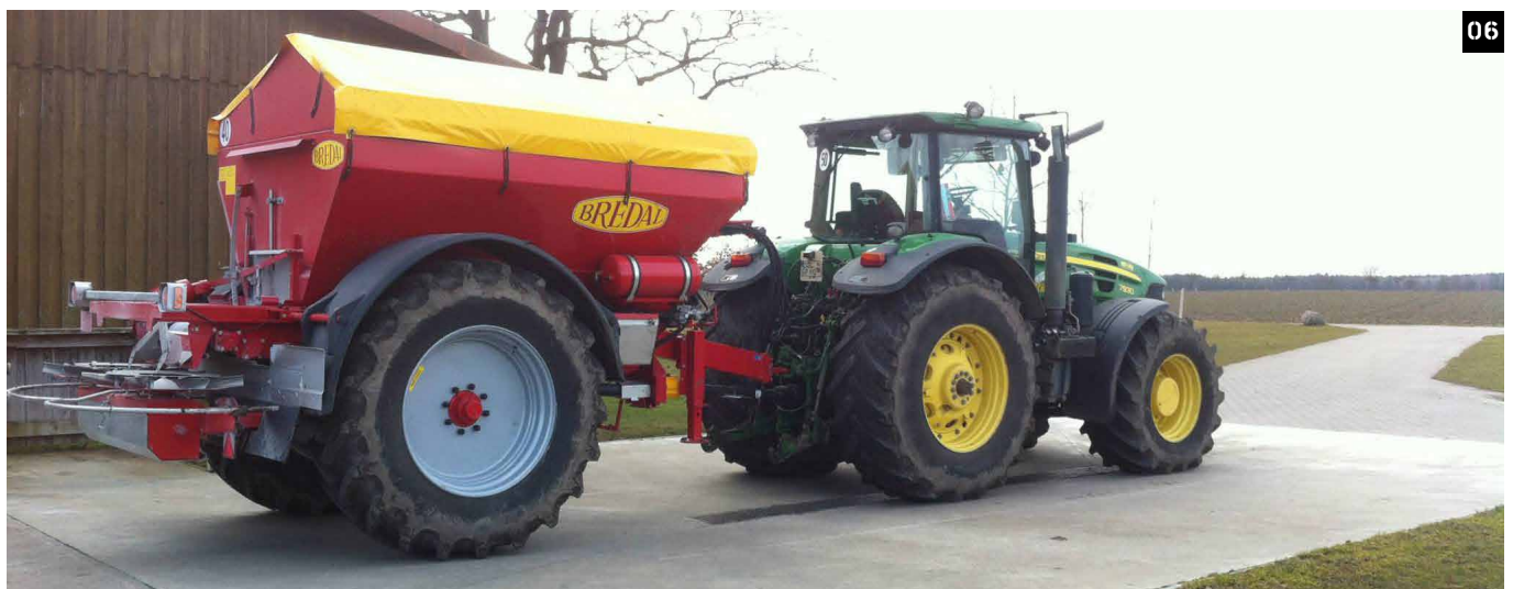
1 > CONSTRUCTION DRAWING SHOWING main components of a K-series spreader 2 > CONVEYOR FRAME IN STAINLESS STEEL with plastic bearings 3 > MECHANICAL GEAR drive dependant dosing 4 > K-SPREADER WITH CHASSIS WHICH IS BOLTED TO THE FRAME 5 > K-SPREADER WITH HIGH CLEARANCE which is welded directly onto the frame 6 > BREDAL K-SPREADER WITH HIGH CLEARANCE (without chassis)
