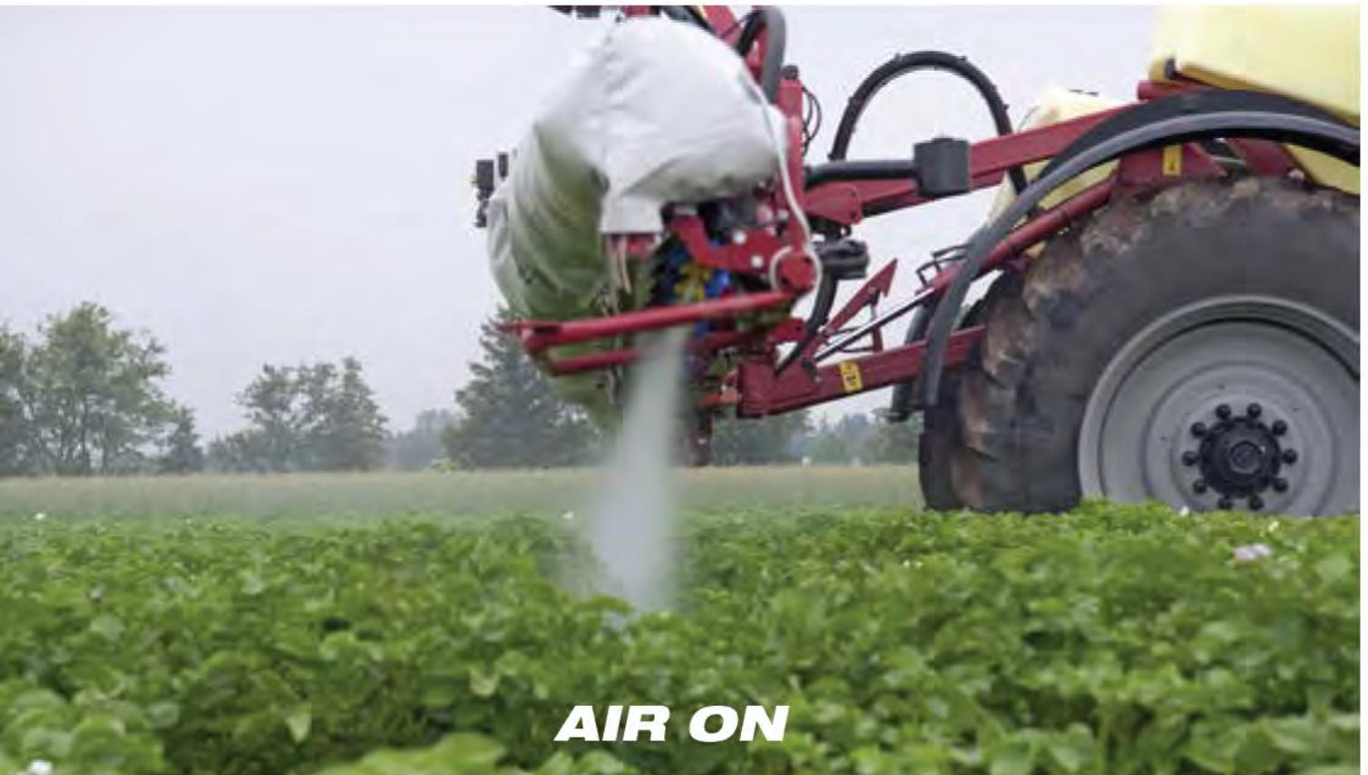
In this situation the wind is about 8-9 m/s, and the drift is strongly reduced with TWIN air on.
