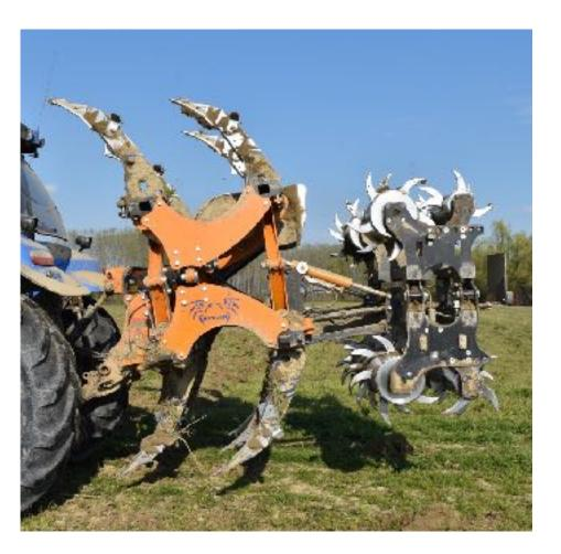
The "SPIDER X" can be used on its own or together with a special double "RCX" roller with hydraulic depth adjustment. The use of a front roller with a diameter of 360mm and a rear roller measuring 220mm, ensures excellent fracturing of the clods and levelling of the soil, avoiding the clogging which typically occurs with smaller diameter rollers.
