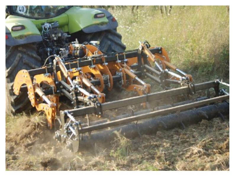
The constructive solution to entrust the delicate task of safeguarding the structure to a battery of accumulators in comparison to a single accumulator, represents an important advantage in terms of reliability. The SPIDER STONE SYSTEM is able to continue to work even in case of failure of one or more accumulators.
