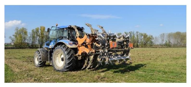
The subsoiler SPIDER X is available in 7, 9 and 11 shank versions. The double 180° folding system allows to reduce to 2.5m the encumbrance for an easier transport. In the operating position, thanks to special safety hooks, the structure is designed to guarantee the maximum rigidity and sturdiness needed for coupling to high-power tractors and for intense and demanding use.
