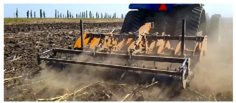
The SPIDER subsoiler range includes the models G,M, and S, with a variable number of shanks: from 5 to 9. The different configurations allow the SPIDER to match tractors with 70 HP up to over 450 HP.
