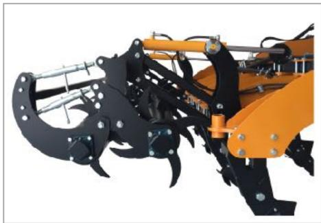
The rollers achieve a preliminary and significant soil tillage, facilitating and reducing the following operations. In addition, the double roller particularly contributes to the mixture of crop residues.
