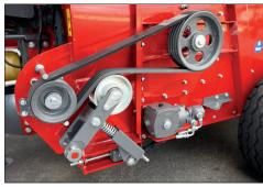
Rotor driven by a very strong 4-groove belt, and with spring belt tensioner.
