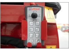
Simple, functional electric control panel with joystick for adjusting the unloading direction and potentiometer for regulating the conveyor belt speed.
