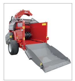
Large loading door allows loading up to two round bales diam.
