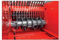
Rotor with 72 knives and with 13 counter-knives for holding the product against the rotor in order to quickly chop all types of fodder and convey it to the turbine, and hydraulic adjustment of the counter-knives to make the rotor more or less aggressive.
