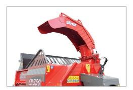
Unloader direction adjustable up to 300° of rotation, and with the possibility of installing the pump kit to spray water on the discharge so as to reduce dust when throwing the product on bedding.
